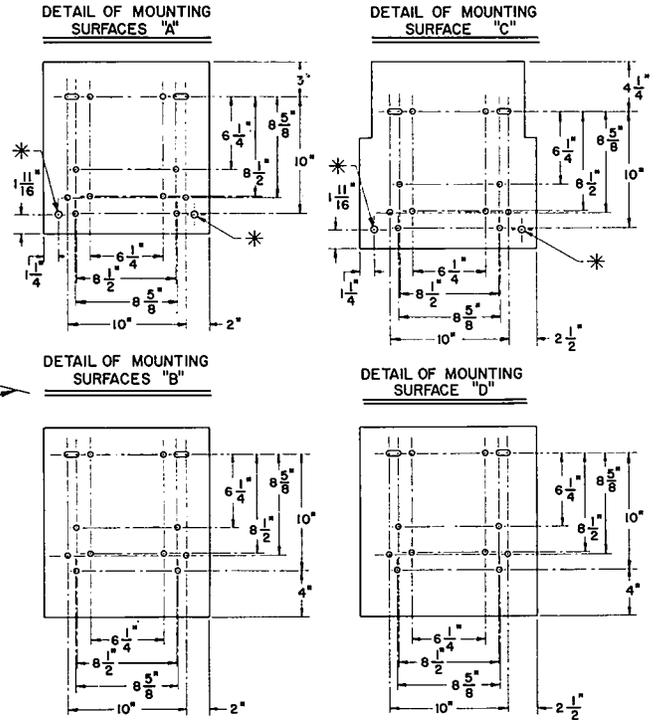
All holes and slots are for 3/8" dia. bolts except those that are indicated by (\*), which are optional arrester mounting locations on surfaces "A" & "C" requiring 1/2" dia. bolts.
